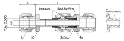
WARNING: A "NO WRENCHING" label is placed on tha hax of the nut in the insulation sections. Do not disconnect at this point. Instructions are provided with every SUPERLOK® dielectric fitting.
