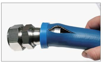
2.Bend hose to expose barbs, then remove hose with a quick pull.
