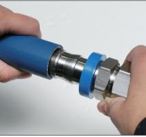
2.Cover first barb of end connention with hose.(Lubrication fitting stem with light oil may ease assembly)
