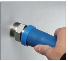
3.Hold end connection against flat surface, Grip hose and push with a steady force until hose seats into blue finshing.
