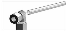
2. With pipe connection tight, the male elbow is pointing in the wrong direction for desired tubing run.
